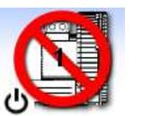
The icon shows a pump unit with the number '1' on its side, a power button symbol at the bottom left, and a red circle with a diagonal slash over the entire symbol.          | <p>Pressing the pump symbol toggles the pump OFF or ON. Message will display PUMP OFF.</p>                                                  |
