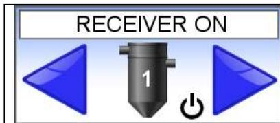
**Receiver Navigation and Status Panel** - This multi-function panel displays messages and receiver status, allows for navigation to each Receiver's configuration screen using the arrow buttons, and allows the receiver to be turned OFF or ON.
