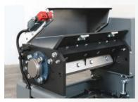
Grinding chamber in 550HV antiwear execution
