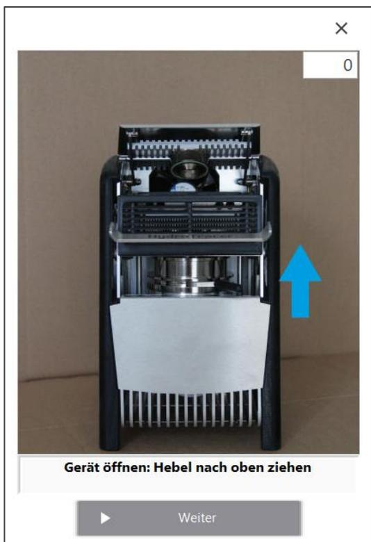
Open the test chamber by pulling the one-hand lever up to the stop. The system fan is switched off.
