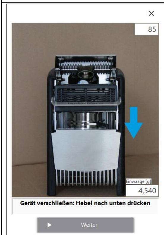
*Close the device by pressing down the one-hand lever. The system fan must now start again. You can start the measurement with "Continue (F10)".*
