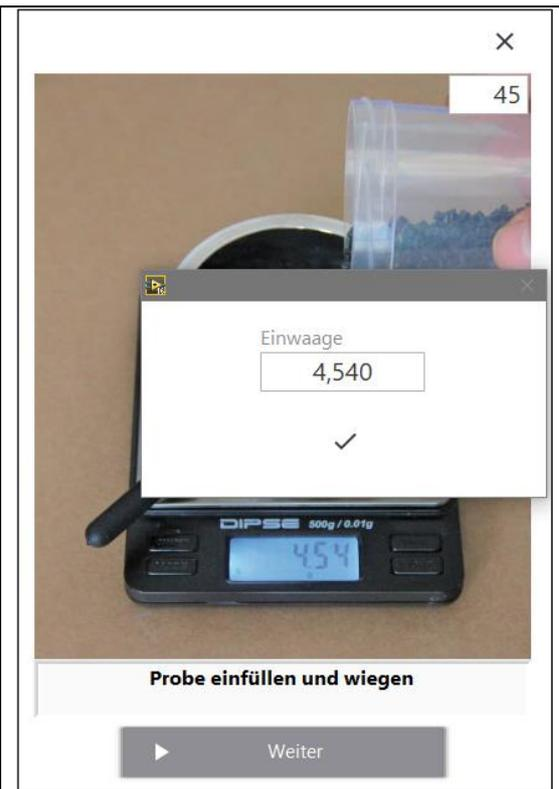
Enter the weight in the input field. Confirm with "✓".
