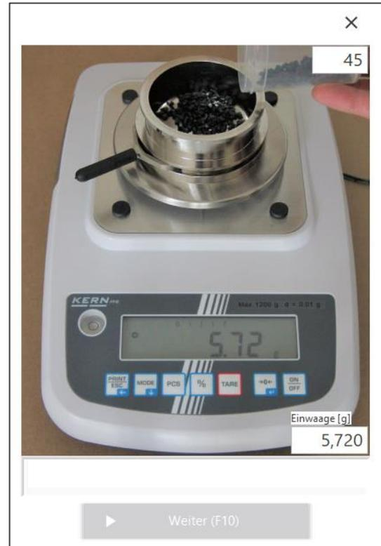
*Send the balance data by pressing the "Print" button. The transmitted weight appears in the "Sample Weight [g]" field.*
