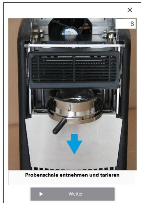
Remove the sample tray. Remove old sample material. Place the sample tray on the scale and tare it.
