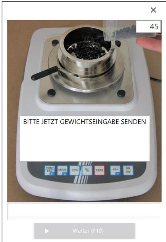
*Place the sample pan on the balance and tare it. Fill in the sample material and spread it until the bottom of the sample cup is evenly covered.*
