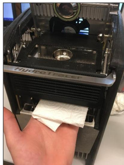
The pipes are cleaned best with a tube brush (see picture). Put in the sample tray to avoid contamination of the heating plate.
